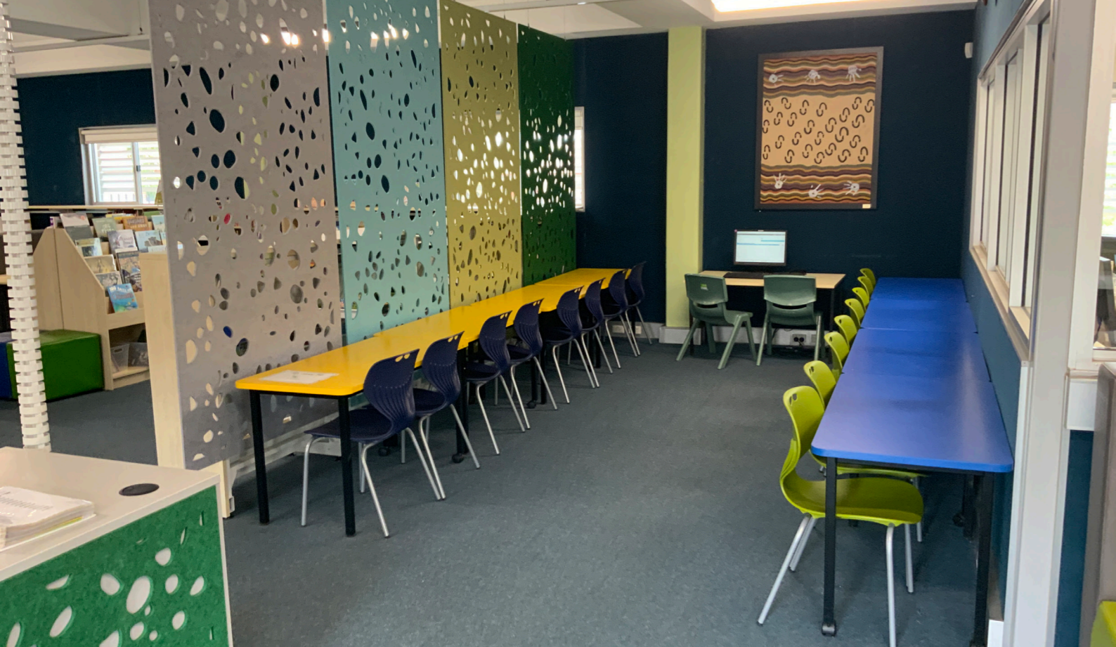
FLOATING SOUND ABSORBERS FROM ACOUSTIC SCREENS WILL HELP REDUCE NOISE
